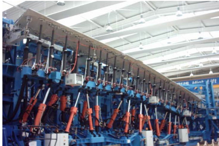
Figure 8: Test rig for flap certification and model validation.
