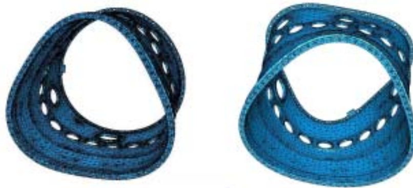
Figure 4: Modes V and IX (triangular deformation front only and front-back with 45 degrees shift).
