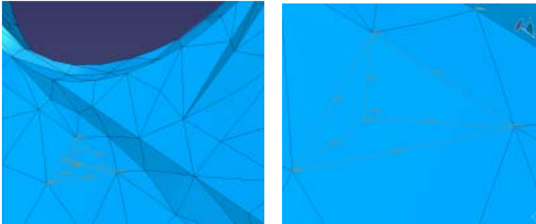
Figure 2: Details of TET10 elements in the mesh (RR Trent 500 COC mesh in LMS Virtual.Lab).
