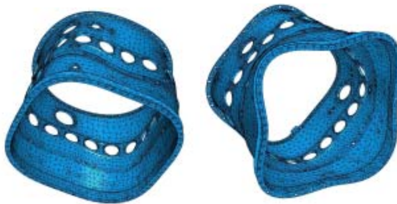
Figure 5: Modes VII and XIII (rectangular deformation front only and front-back with 45 degrees shift).
