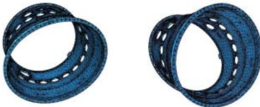
Figure 3: Modes I and III (“Pumping” front only and front-back with 45 degrees shift).
